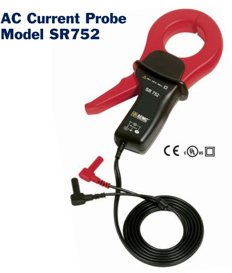
The Model SR752 is designed for use in industrial and utility environments. The unique ergonomic design allows it to easily clamp onto cables or small bus bars. It is built to the highest safety and performance standards including the CE Mark and is UL approved for Canada and United States.
