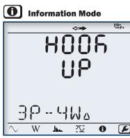
Hook up, voltage and current ratios and aggregation period can be configured from the front panel of the PEL 103.
