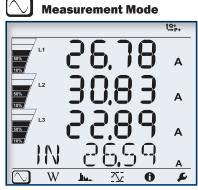
Real-time updates are displayed for voltage, current, power, frequency, power factor and tangent.
