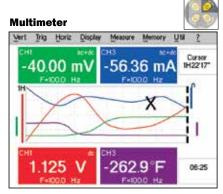
Automatic recording of the measured values are stored in memory on all active channels allowing review of periods lasting from five minutes to 24 hours.
