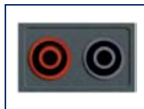
Jacks: Two standard safety banana jacks (4mm)
