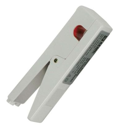
Small, compact and very tough, the Model MN185 is designed for measurements from 50mA to 120AAc. The "clothes pin" shape makes it ideal for use in tight areas, such as breaker panels, controller panels or outlets. It is an excellent companions to all DMMs.
