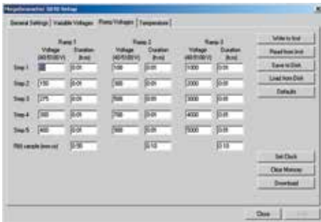
Model 5070 includes Ramp Function which allows programming of three different ramp test profiles, each containing up to five voltage steps between 40 and 5100V and time per step of up to 10 hours.
