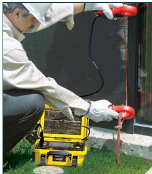
The Model 6471 provides a fast and easy way to measure the value of the earth/ground using the 2 Clamp method (no auxiliary rods needed).
