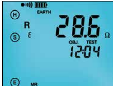
Memory Recall displays test results stored at a specific memory location.
