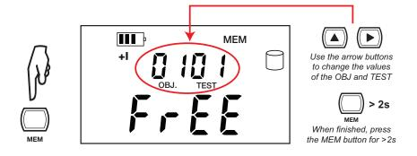
**6.** If the user selects a memory address that is already occupied, **all** appears on the main screen. To overwrite the location, press the **MEM** button for >2s.
