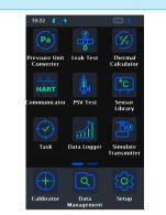
The onboard applications provide a useful selection of features including HART communicator, high static differential pressure mode, pressure leak test, safety valve test, analog transmitter calibration, unit converter, thermal calculator, and snapshots to name a few.
